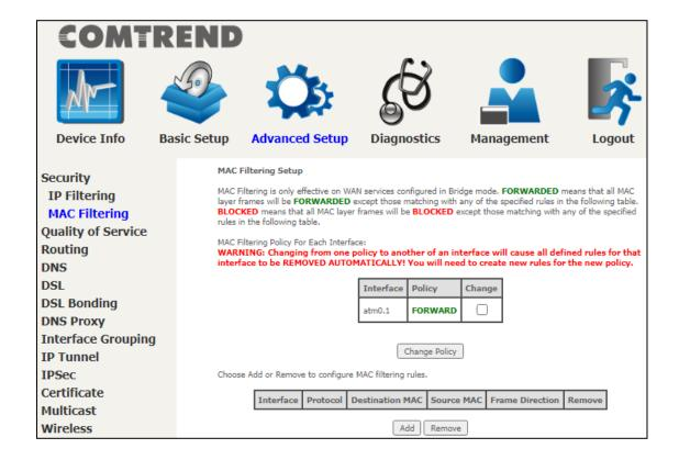
Choose **Add** or **Remove** to configure MAC filtering rules. The following screen will appear when you click **Add**. Create a filter to identify the MAC layer frames by specifying at least one condition below. If multiple conditions are specified, all of them must be met.
