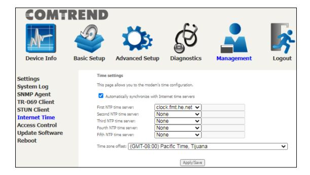
**NOTE:** Internet Time must be activated to use. See 5.5 Parental Control. The internet time feature will not operate when the router is in bridged mode, since the router would not be able to connect to the NTP timeserver.
