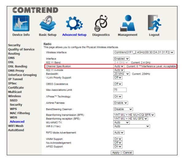
3. Both devices need to have a (different) fixed access SSID (Network Name). See section 6.13.1 SSID for details.
