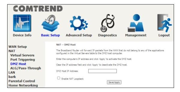
To **Activate** the DMZ host, enter the DMZ host IP address and click **Save/Apply**.
