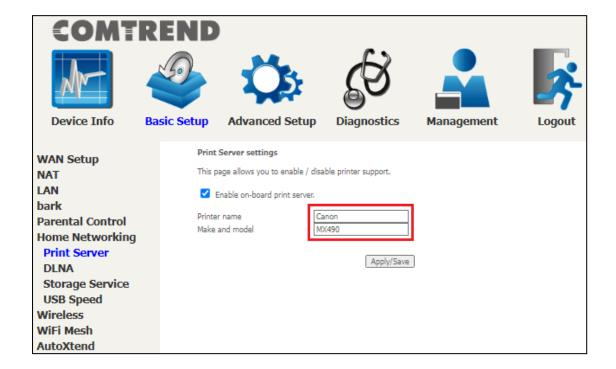
**NOTE**: The **Printer name** can be any text string up to 40 characters. The **Make and model** can be any text string up to 128 characters.
