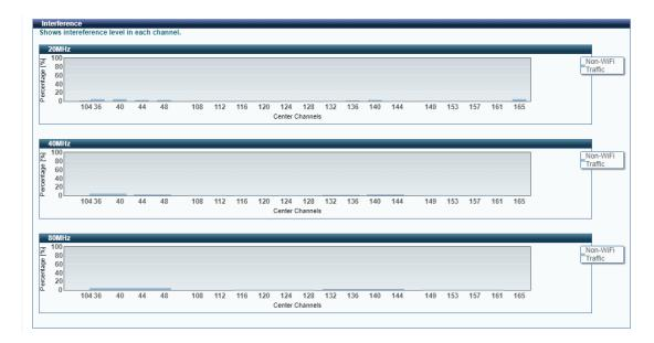
Shows the highest RSSI (Received Signal Strength Indicator) on each adjacent channel. Adjacent AP and associated stations are displayed for checking interference on those channels.
