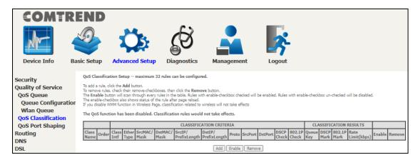
Click **Add** to configure a network traffic class rule and **Enable** to activate it. To delete an entry from the list, click **Remove**.
