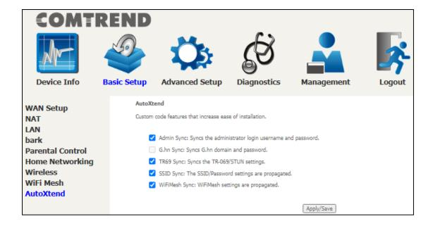
To enable the AutoXtend features, check the required checkboxes and click the **Apply/Save** button.
