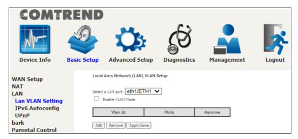
To enable VLAN Mode, check the checkbox and click the **Apply/Save** button. Click the **Add** button to display the following.
