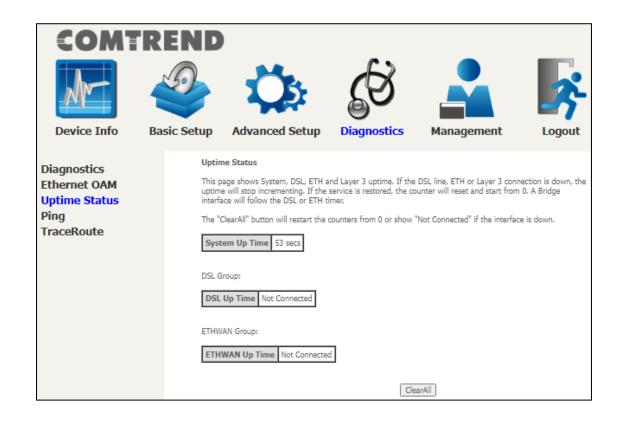
The "ClearAll" button will restart the counters from 0 or show "Not Connected" if the interface is down.
