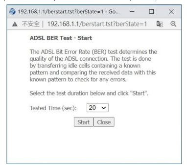
Click **Start** to start the test or click **Close** to cancel the test. After the BER testing is complete, the pop-up window will display as follows.
