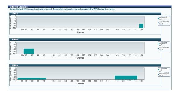
For each AP, the graph shows the control channel and extension channels. Extension channel is any channel spanned by the AP that is not a control channel.
