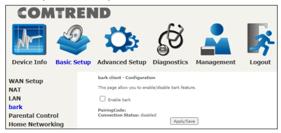
**Step 1**: Check the checkbox and click the **Apply/Save** button to enable this feature.
