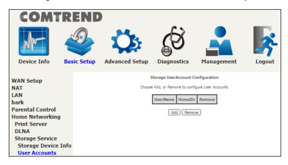
Click the **Add** button to display the following. volumeName would be disk1\_1 if only 1 USB has been plugged into the device.
