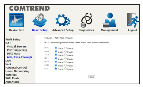
To allow/deny the corresponding ALG protocol, select Enable / Disable and then click the **Save** button. After reboot, the protocol will be added/removed to/from the system module.
