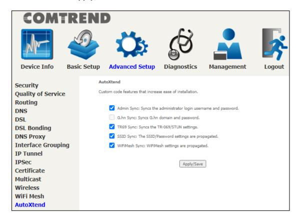
To enable the AutoXtend features, check the required checkboxes and click the **Apply/Save** button.
