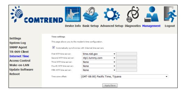
**NOTE:** Internet Time must be activated to use 5.5 Parental Control. In addition, this menu item is not displayed when in Bridge mode since the router would not be able to connect to the NTP timeserver.
