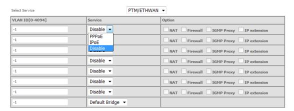
**WAN services list for PTM/ETHWAN mode:** A maximum of 7 WAN services with corresponding VLAN ID (-1 indicates no VLAN ID is required for the service) are required to be configured for ADSL/VDSL PTM mode and ETHWAN. The services will be detected in order. Users can modify the 7 pre-configured services and select **disable** to ignore any of the services to meet their own requirements and also reduce the detection cycle.
