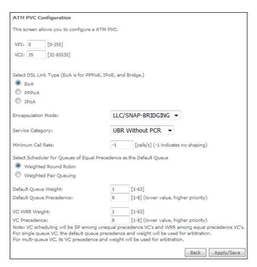
There are many settings here including: VPI/VCI, DSL Latency, DSL Link Type, Encapsulation Mode, Minimum Cell Rate, Service Category, Connection Mode and Quality of Service.
