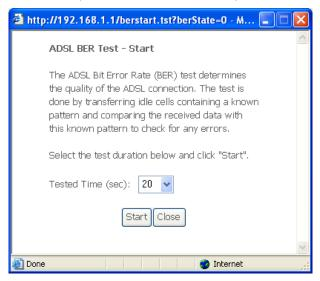
Click **Start** to start the test or click **Close** to cancel the test. After the BER testing is complete, the pop-up window will display as follows.
