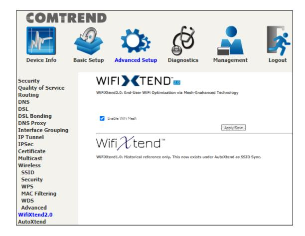
To enable the end-user WiFi optimization via mesh-enhanced technology, check the checkbox and click the **Apply/Save** button.
