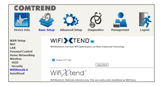
To enable the end-user WiFi optimization via mesh-enhanced technology, check the checkbox and click the **Apply/Save** button.
