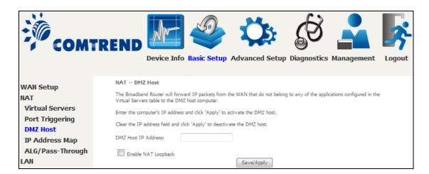
To **Activate** the DMZ host, enter the DMZ host IP address and click **Save/Apply**.
