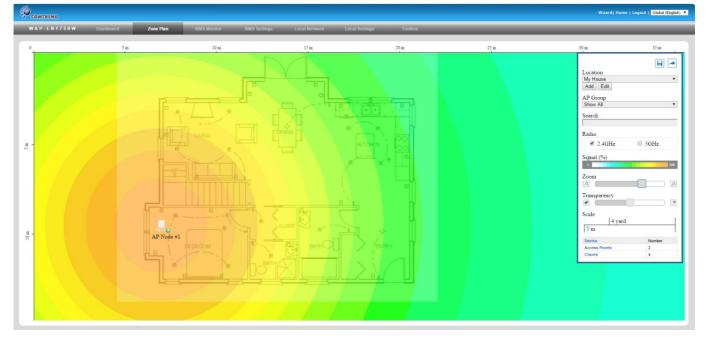
**Zone Plan** displays a customizable live map of Managed APs for a visual representation of your network coverage. Each AP icon can be moved around the map, and a background image can be uploaded for user-defined location profiles using **NMS Settings**  $\rightarrow$  **Zone Edit**. Options can be configured using the menu on the right and signal strength is displayed for each AP. (Available settings will vary depending on the device being used as an AP Controller.)
