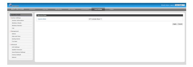
**Local Settings** are for your AP Controller. You can set the operation mode and view network settings (clients and logs) specifically for the AP Controller, as well as other management settings such as date/time, admin accounts, firmware and reset. (Available settings will vary depending on the device being used as an AP Controller.)
