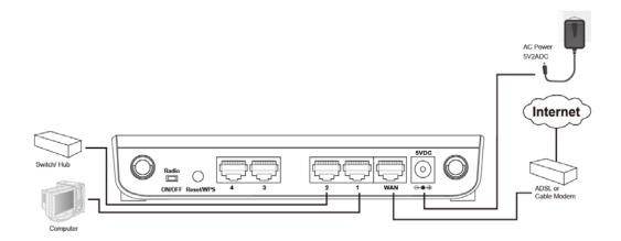
4. Check all LEDs on the front panel. The 'Power' LED should be steadily on, WAN and LAN LEDs should be on if the computer / network devices connected to the respective port of the router is powered on and correctly connected. If the Power LED is not on, or any LED you expected to be on is not on, recheck the cabling, or jump to '4-2 Troubleshooting' for possible reasons and solutions.
