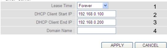
These settings are only available when the 'DHCP Server' in the 'LAN IP' section is 'Enabled', and here are descriptions of every setup item:
