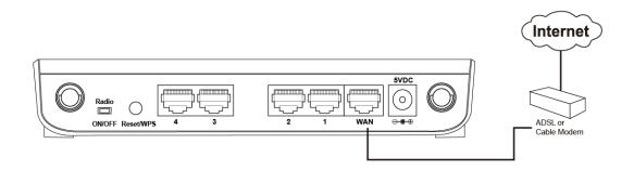
2. Connect your computers and network devices (network-enabled consumer devices other than computers, like game consoles, or a switch / hub) to an available LAN port of the router.
