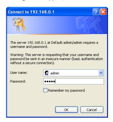
Input the user name and password in their respective fields, the default user name is 'admin', and the default password is 'admin', then press the 'OK' button, and you can see the Quick Setup interface of this router:
