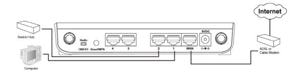
3. Insert the A/C power adapter into the wall socket, and then connect it to the 'Power' socket of the router.
