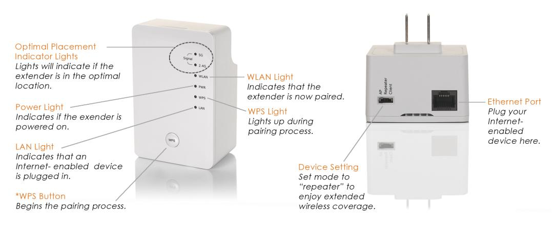
\* If you wish to reset the extender to factory default settings (clear all settings), press and hold the "WPS" button for 10 seconds.
