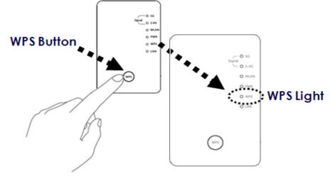
3. Within 2 minutes, go to your wireless router/gateway/access point and press the **WPS Button** for 2 seconds.
