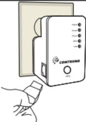
Connect your computer and Wireless-N Range Extender by Ethernet cable.
