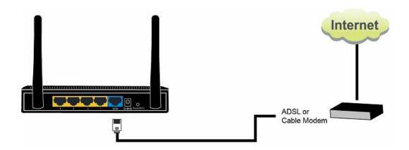
2. Connect your computers and network devices (network-enabled consumer devices other than computers, like game consoles, or a switch / hub) to an available LAN port of the router.
