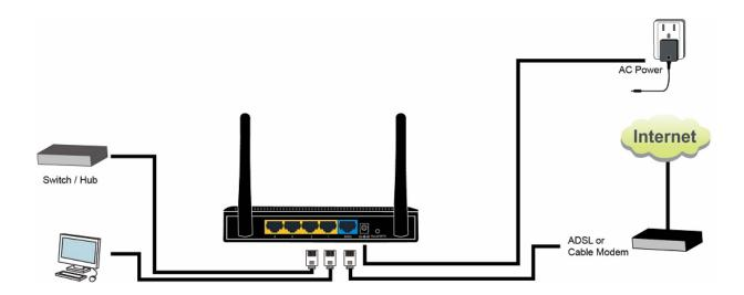
4. Check all LEDs on the front panel. The 'Power' LED should be steadily on, WAN and LAN LEDs should be on if the computer / network devices connected to the respective port of the router is powered on and correctly connected. If the Power LED is not on, or any LED you expected to be on is not on, recheck the cabling, or jump to '4-2 Troubleshooting' for possible reasons and solutions.
