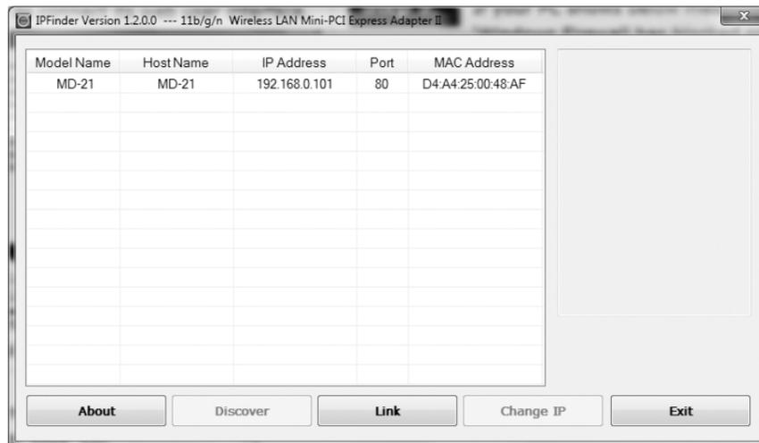
2. If you need to change the camera's IP address, click 'Change IP' button on your selected camera to change the camera's IP address.
