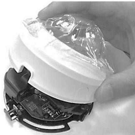
7. Make sure to keep the network camera cover closed and the network cable fed out the desired path.
