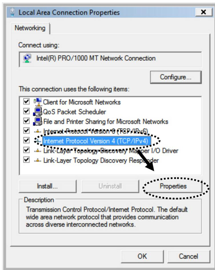
2. Select 'Obtain an IP address automatically' and 'Obtain DNS server address automatically', then click the 'OK' button.
