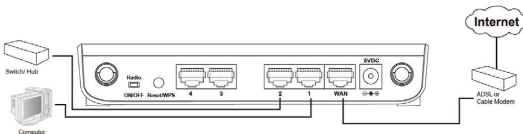
3. Insert the A/C power adapter into the wall socket, and then connect it to the 'Power' socket of the router.
