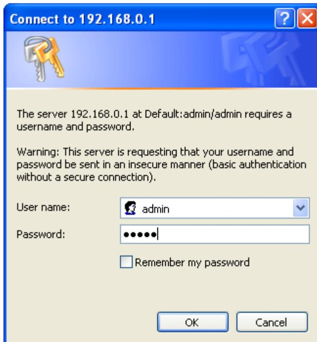
Input the user name and password in their respective fields, the default user name is '**admin**', and the default password is '**admin**', then press the 'OK' button, and you can see the Quick Setup interface of this router:
