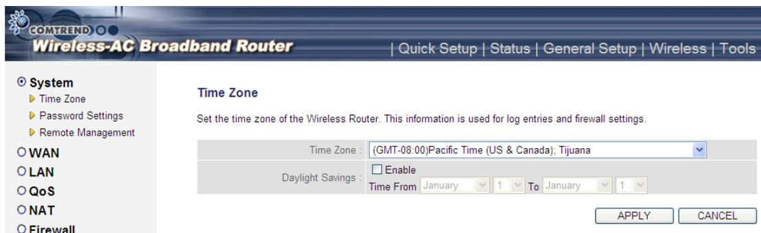
Select the time zone from the 'Set time zone' drop-down list, and input the IP address or host name of the time server. If you want to enable the daylight savings setting, check the 'Enable Function' box, and set the duration of daylight setting. When you finish, click the 'Apply' button. You'll see the following message displayed on the web browser:
