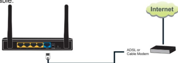
2. Connect your computers and network devices (network-enabled consumer devices other than computers, like game consoles, or a switch / hub) to an available LAN port of the router.
